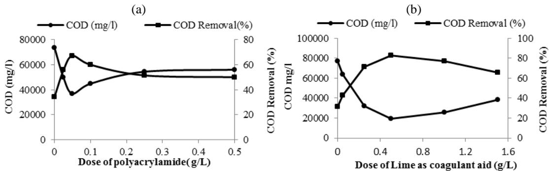
Figure (3): Coagulation/Precipitation process using alum (a) Determination of optimum dose of polyacrylamide, (b) Determination of optimum dose of lime at 1.5g/L alum dose.
