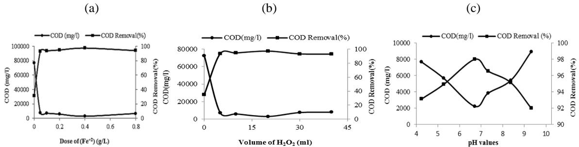
**Figure(4):** Fenton reaction after alum-lime (a) Determination the optimum dose of Fe<sup>2+</sup>, (b) Determination the optimum volume of H<sub>2</sub>O<sub>2</sub> ml at 0.4 g/L Fe<sup>2+</sup>, (c) Determination the optimum pH at 0.4 g/L Fe<sup>2+</sup> and 20 ml of H<sub>2</sub>O<sub>2</sub> (30%).
