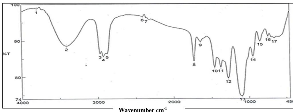
Figure (1): Infra-Red spectrophotometer of ergosterol-propyl ester.
