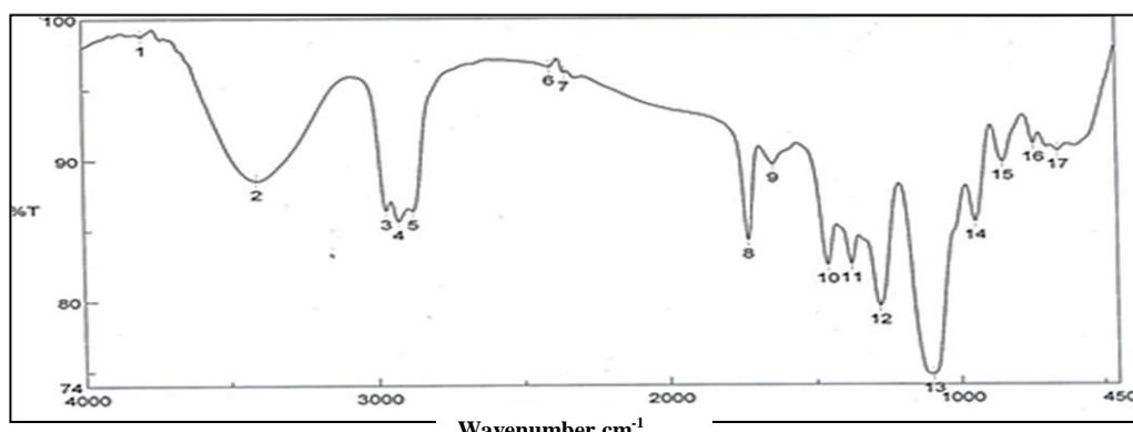
**Figure (1):** Infra-Red spectrophotometer of ergosterol-propyl ester.
