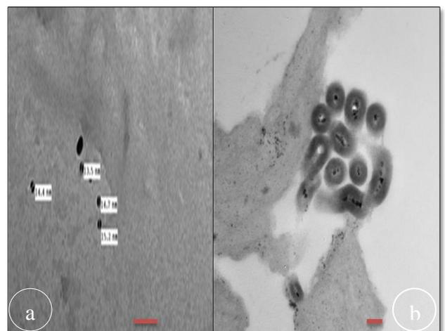
**Figure (5b)** Transmission electron microscopy (TEM) images of (a) Iron oxide nanoparticles (IONPs) ( $\text{Fe}_3\text{O}_4 + \text{Fe}_2\text{O}_3$ , diameter in mean =  $15.2 \pm 2.6$  nm), and (b) CH-MNPs immobilized cellulase. Where the scale bar = 100 nm.
