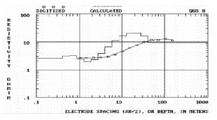
Figure (5): Example of an interpreted VES curve for VES No. 8 according to Zohdy and Bisdorf method (1989).
