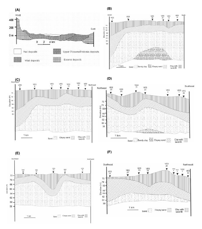
Figure (6): (A) Lithological cross section in the Nile Valley at Luxor (modified after Said, 1981). (B, C, D, E, and F) Geoelectrical cross sections P1, P2, P3, P4, and P5.
