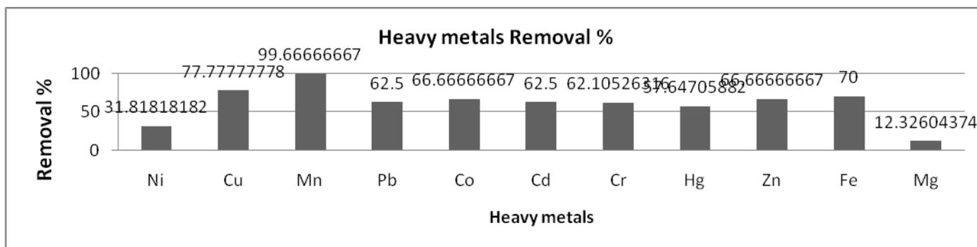
**Figure (1):** Removal measurement of heavy metals in the aerated lagoon system in Ismailia, Metals removal ratio by free and immobilized cells of bacterial strains.
