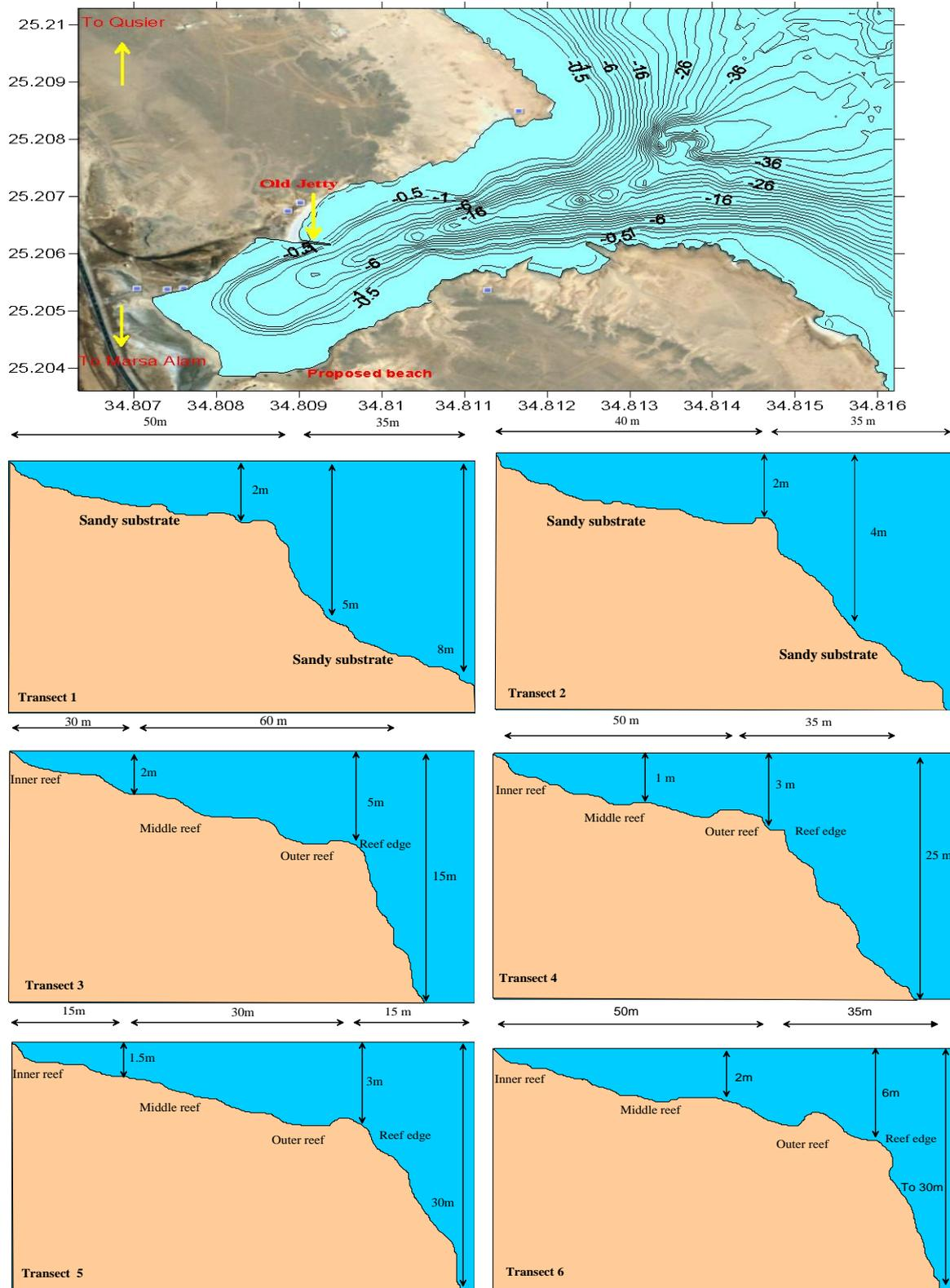
Figure (2): Bathymetric map and cross section of six sectors at Gabal El-Rosas Reefs, Red Sea.
